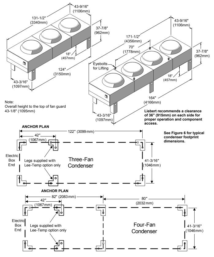
Figure 4 Condenser planning dimensional data—Three-fan and four-fan units
